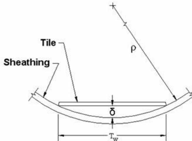
Figure 4 - Exaggerated View of Curvature of Wood Subfloor beneath Tile Covering
