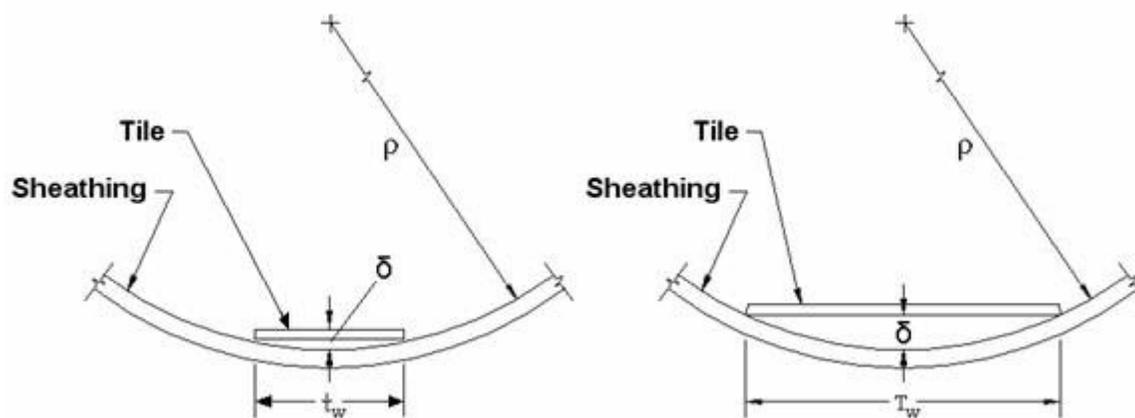
Figure 5 - Sensitivity to Curvature Increases with Tile Format
