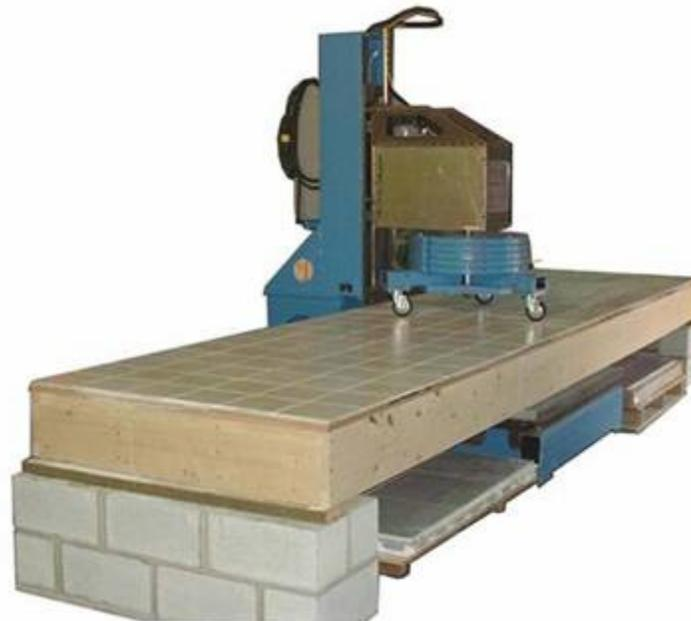
Figure 3a - Universal Floor Tester Full-Scale Assembly
