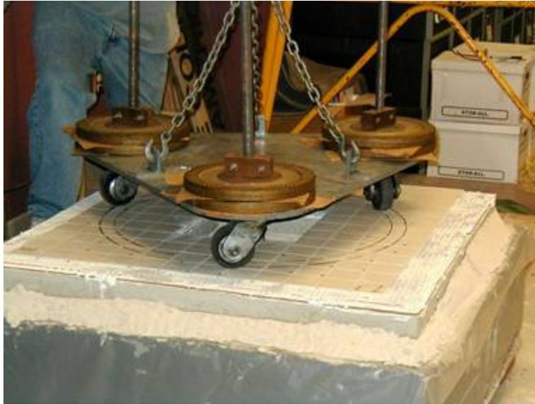
Figure 1 - Robinson-Type Floor Tester
