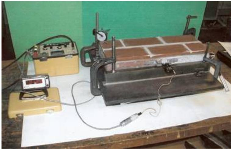
Figure 2 - System Crack Resistance Tester
